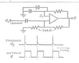
This circuit is identical to (3.6) except that a diode has been shunted across the capacitor permitting  $e_e$  to vary in only one direction with respect to ground and resulting in a "single shot" multivibrator. Thus for the direction shown, a positive trigger will produce positive pulses, whose duration, as before, depends on RC and  $\Delta$ . The polarity may be reversed by reversing the diode and using negative pulses.
