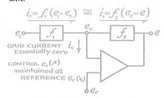
When  $e_r$  is grounded,  $e_c$  becomes zero. If, moreover, the perfectly general functional relations  $f_1$  and  $f_2$  became the linear operational impedances  $Z_1$  (p) and  $Z_2$  (p), respectively, there results the well-known fact:
