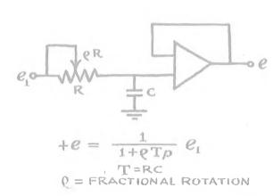
A non-inverting first order lag with low distortion and without attenuation is provided by this positive input application.
