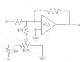
By shifting the biasing circuit to the negative side in the form of a constant adder, the plus input, although shown ground, becomes generally available.
