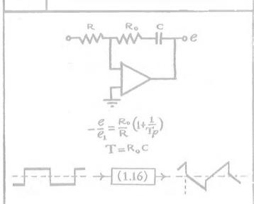
When a resistance R, is added to the feedback capacitor of the Integrator (1.8), the circuit will transmit the input signal modified by the addition of the time integral of the input.
