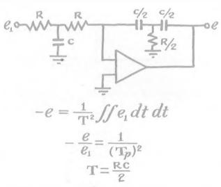
Another extension of Circuit (1.8) permits a single amplifier to generate the second time integral of an input signal. This element is sometimes useful for handling dynamic system equations such as
