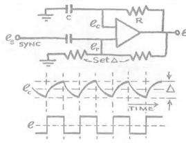
By arranging the circuit (3.5) to provide its own trigger signal, a "free-running" multivibrator results. As the control voltage,  $e_e$ , rises past the hysteretic reference,  $e_r$ , the output drops abruptly to its negative value, causing  $e_e$  to begin to drop. This sequence is then repeated alternately negative and positive. Provision of the sync input allows the oscillator to be locked into phase with any other signal.
