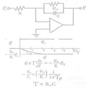
A first order "lagging" or tardigrade operation is performed by this circuit containing a parallel  $R_{\text{o}}C$  network in the feedback path. Variation in  $R_{\text{o}}$  will produce proportional changes in both gain and time constant.
