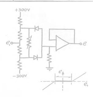
This application of the Dwell Circuit (4.4) will yield a device providing a fixed but adjustable inert zone within which an input signal  $e_1$  results in a zero output signal e. Outside this threshold, response will follow stimulus.
