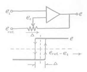
The addition of a potentiometer (or fixed resistances) connecting the output back to the reference, provides a two-valued control voltage,  $e_c$ , to the operational amplifier. When the output, e, is full positive, the control,  $e_c$ , is higher than when e is full negative. This shift in effective reference introduces hysteresis or "free-play", in an amount proportional to potentiometer drop, $\Delta$ .
