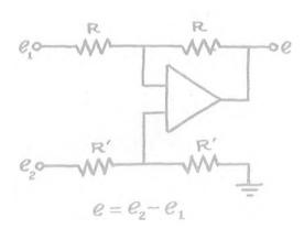
A modification of Circuit (2.2) permits direct subtracting operations. The input signal,  $e_1$ , is thus inverted and deducted from the other input,  $e_2$ .
