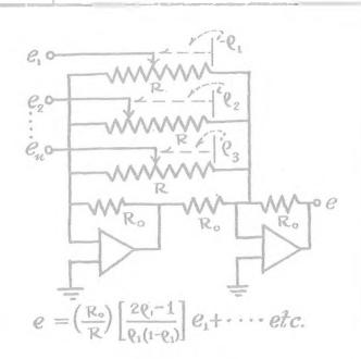
A fully adjustable linear combinor is formed as indicated using two amplifiers. Mid-setting of each potentiometer gives zero influence coefficient, while full scale traverse ranges from  $-\infty$  to  $+\infty$ .
