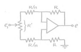
By driving the two inputs of the Subtractor (2.3) from a potentiometer, a variable gain device is produced which has certain advantages, particularly for empirical adjustments requiring a small range of gain each side of zero.
