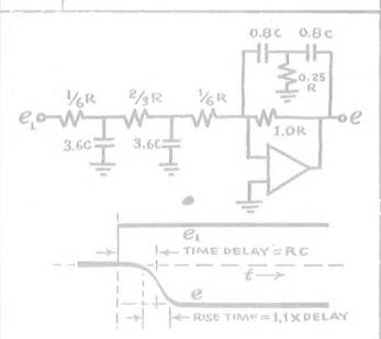
A unit gain phase shift or transmission delay is approximated by this circuit, with non-overshooting response as indicated.
