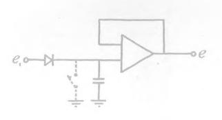
This circuit consisting of a diode connected so that a condenser may be charged but not readily discharged, when driven by a load impedance source and followed by an amplifier used as a voltage reproducer, will provide an output voltage which is the peak value over a past history of the input. This epoch may be varied through manipulation of the size and discharge conditions of the capacitor (i.e. shunt resistance or switch).
