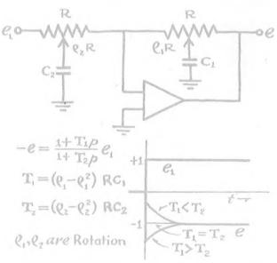
Using the previous input circuit also in the feedback path produces a leading or lagging action depending upon the relative weights of  $T_1$  and  $T_2$ . This circuit is useful as a "lead-lag" compensating element in instruments and controllers. It also has many applications in the representation of thermal systems.
