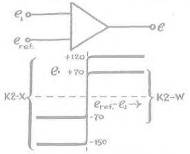
The operational amplifier, by itself, serves as a sensitive voltage detector. When the input voltage,  $e_1$ , changes but a few millivolts up or down from a fixed or variable reference voltage,  $e_{\rm ref}$ , the output, e, will swing from either -150 to  $+120{\rm VDC}$  (for the K2-X) or -70 to +70 VDC (for the K2-W). If  $e_{\rm ref}$  is zero, one thus obtains a "flip-flop" or two-position contactor.
