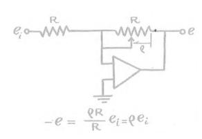
If the potentiometer is placed in the feedback path alone, a proportioning device is obtained with narrower range than that of (1.5), but having a linear scale with respect to potentiometer rotation.
