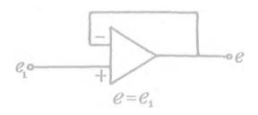
The simplest use of the positive input for a variable signal,  $e_1$ , is as a voltage reproducer or follower. Here the output,  $e_i$ , is fed back into the negative input as degenerative feedback at high gain.
