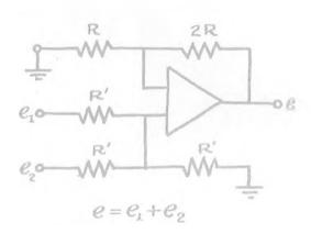
An example of advantageous use of both inputs is afforded by the circuit shown. The output, e, is the direct, positive sum of the two inputs,  $e_1$ , and  $e_2$ .
