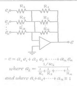
A special case of the Linear Combinor (1.3) utilizes matching resistors in a voltage-dividing network which assures that the sum of the weighting coefficients is always precisely unity. This yields an output which is the inverted weighted average of the inputs.
