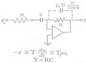
This circuit produces the time derivative of the input signal,  $e_1$ . The small shunt capacitor  $C_1$  serves to prevent oscillation in certain applications and does not introduce critical error. It may also sometimes be necessary to add a small resistor  $R_1$ , in series with the input capacitor.
