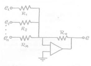
$$-e = \left(\frac{R_o}{R_1}\right)e_1 + \left(\frac{R_o}{R_2}\right)e_2 + \cdots + \left(\frac{R_o}{R_n}\right)e_n$$
