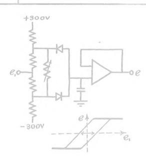
If a small Capacitor replaces the shunt resistor of the previous circuit, an adjustable hysteretic effect will result. This yields the response associated with free play or loose joints in gears or linkages, as well as similar phenomena in biomechanics and physics.
