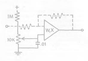
This circuit avoids the use of biasing cells, and is useful where the plus input is not needed.
