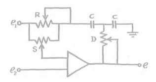
This ingenious circuit permits a single amplifier to provide signal transformation for feedback control of a measured variable, in the form of a scaled voltage  $e_2$ , arising in any manufacturing process guidance system, and the like.
