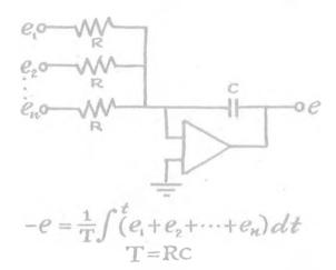
By providing a multiplicity of input resistors, the Circuit (1.8) is generalized to a Summing Integrator.
