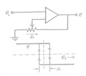
Here the reference voltage,  $e_{\rm ref}$ , of circuit (3.2) is grounded. The performance is identical in character, but now the device becomes a simple hysteretic contactor, extremely useful for control and instrumentation purposes, where stable, two-position operation is desired. The value of  $\Delta$  in these applications often becomes a necessary or desirable control parameter.
