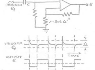
If the circuit (3.3) is AC coupled to a pulsed trigger voltage, a bistable controlled multivibrator results. In the absence of trigger pulses the output will remain in its last state. But upon receipt of a positive pulse, the output will swing full negative and vice versa. By varying the value of the threshold,  $\Delta$ , the circuit can be selective with respect to pulse height.
