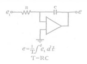
An operational amplifier with capacitance feedback and resistive input will provide the inverted time integral one of the input voltage signal.
