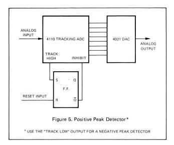
The Model 4110's TRACK HIGH and TRACK LOW outputs are the key to this circuit. The 4110 is an inverting ADC, i.e., as the input goes negative the digital output is increasing toward all "ones." When the input goes positive, therefore, we get a TRACK LOW pulse for every count pulse. The instant the input signal starts to turn around, a TRACK HIGH pulse appears and inhibits any further change. To repeat the operation, hold the flip flop in reset for approximately 30  $\mu$ sec.
