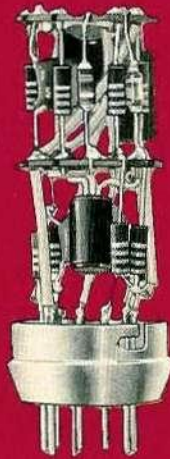
Typical T-Series construction details, actual size.
