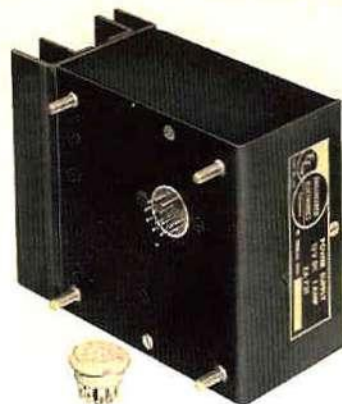
Model ZA-721 transistorized 12-volt DC, 1-Amp Regulated Power Supply plugs into modified 14-pin miniature tube socket. Seated height is identical with T-Series plug-in circuit package (2-3/16").
