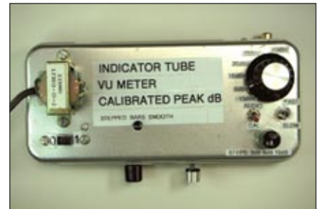
PHOTO 3: Top view of dB step generator and VU meter. a) output offset control to adjust start of deflection. b) output gain control to adjust maximum deflection. c) VU display mode; stepped bars over blank background or smooth bars over stepped background. d) power switch and LED power-on indicator.
