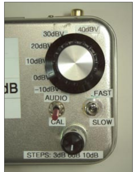
PHOTO 4: Step generator controls. a) input attenuator. b) calibration switch. c) decay: 6dB/sec or 6dB/100ms. d) dB step size. e) phono jack audio input. f) submini jack dB step output.
