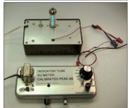
PHOTO 5: dB step generator and VU meter driving EM84 fixture.
