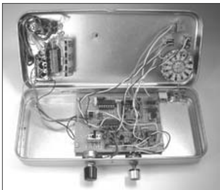
PHOTO 6: Interior of dB step generator and VU meter, with power supply on the left side of the lid and input attenuator on the right. Output offset knob on the lower left and the output gain knob on the lower right.
