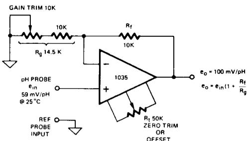
Figure A. pH Measurement Circuit
