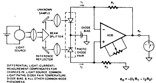
Figure C. Differential Reflectometer
