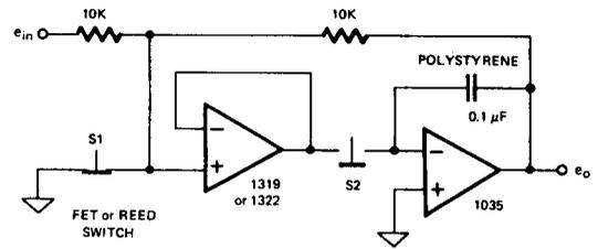
Figure B. Integrating Sample & Hold (Shown in Hold)
