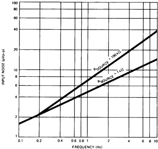
**Figure 2. Equivalent Input Noise vs Closed Loop Bandwidth vs Source Impedance**
