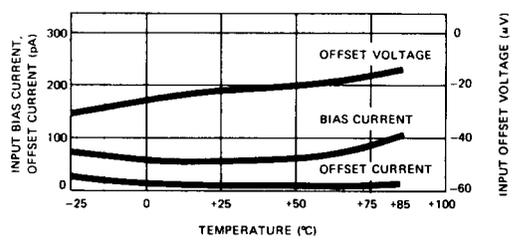
**Figure 3. Typical Input Characteristics vs Temperature**
