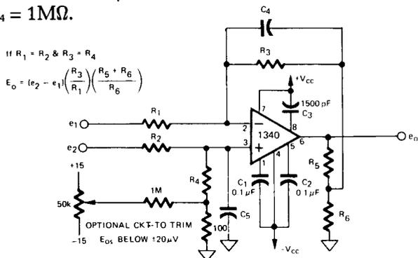
Figure 1. 1340 Connected as Differential Amplifier
