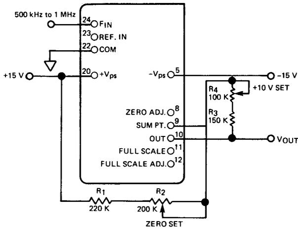
Figure 10. Output Offset and Expansion to Provide 0 to +10 V Output for 500 kHz to 1 MHz F<sub>in</sub>
