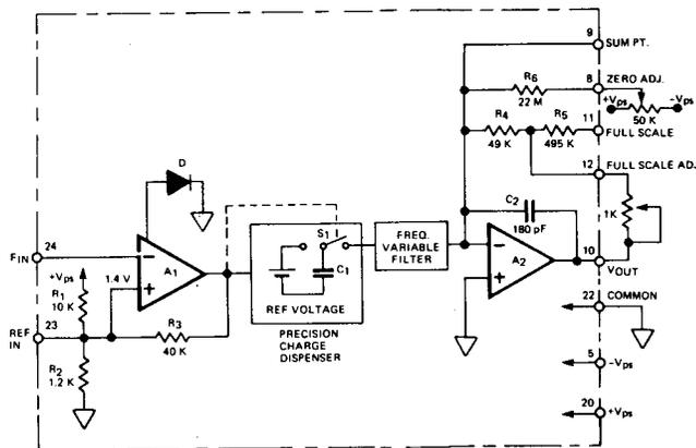
Figure 1. F to V Simplified Block Diagram
