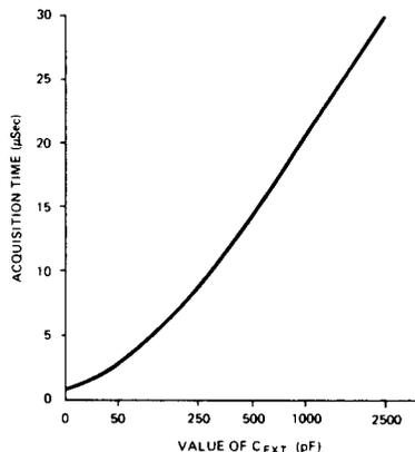
Figure 3. Effect of External Capacitance on Acquisition Time
