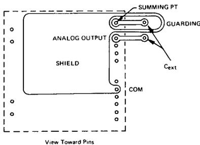
Figure 2. Shielding & Grounding
