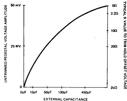
Figure 4. Pedestal Voltage and Trim R vs. External Capacitance
