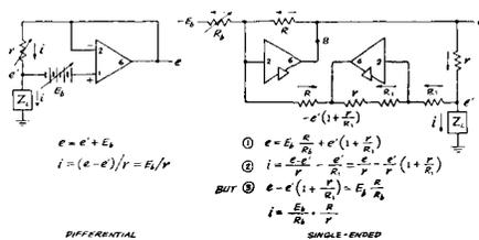
Fig. 1—Driving current to a grounded load.
