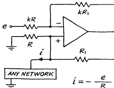
Fig. 2—Differential operational amplifier as current injector.
