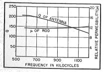
FIG. 3—Variation of Q of antenna and permeability of rod with frequency
