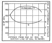
FIG. 1—Variation in Q of coil and permeability of ferrite rod with position of coil on rod
