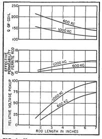
FIG. 2—Variation of Q of coil, permeability of ferrite rod and voltage pickup of antenna with rod length
